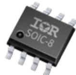
AUIRS2301S Fast MOSFET driver IC
