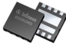
BSZ0910ND Half-bridge in PQFN 3.3 x 3.3 package
