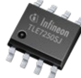
TLE7250SJ CAN transceiver
