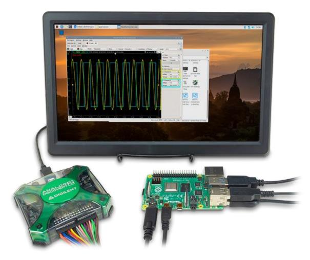
The Analog Discovery 2's WaveForms software is Mac, Windows, and Linux compatible, and also has a version for ARM. It works on devices such as the Zybo, Beaglebone Black, and Orange PI PC, but unfortunately, due to an issue with the FTDI driver on older versions of Raspberry Pi, the ARM version of WaveForms has not worked on Raspberry Pi with Analog Discovery 2. That all changed when RPi 4 was released!
