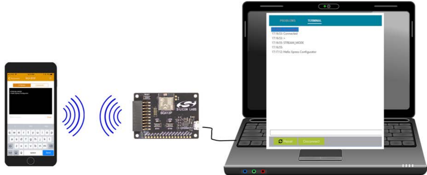
Figure 2: OTA support for the BGX module is offered out of the box with the BGX commander mobile application. This allows for remote configuration of Bluetooth capabilities regardless of the type of smartphone being utilized.
