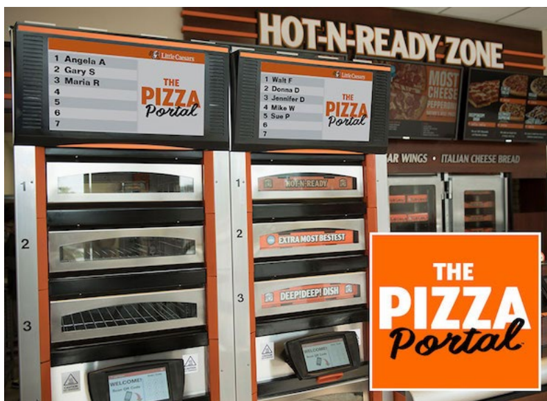
Figure 1 – The Apex “Pizza Portal” includes multiple HMIs. Rear- and forward-facing HMIs for kitchen and service personnel to interact with the portal and a large, high-up customer-facing HMI that displays order status, advertisements, and other useful information.
