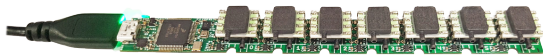
HSC or RSC Series, DIP package, dual ported pressure sensors on a Pressure Sensor Interface Card.
