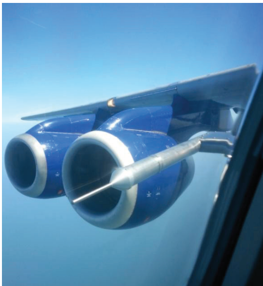
Digital Seven Hole Probe System shown mounted on an NCAS FAAM BAe146 atmospheric measurement aircraft as part of its air data calibration system. This system is also the smallest UAV (Unmanned Aerial Vehicle) air data system currently available.
