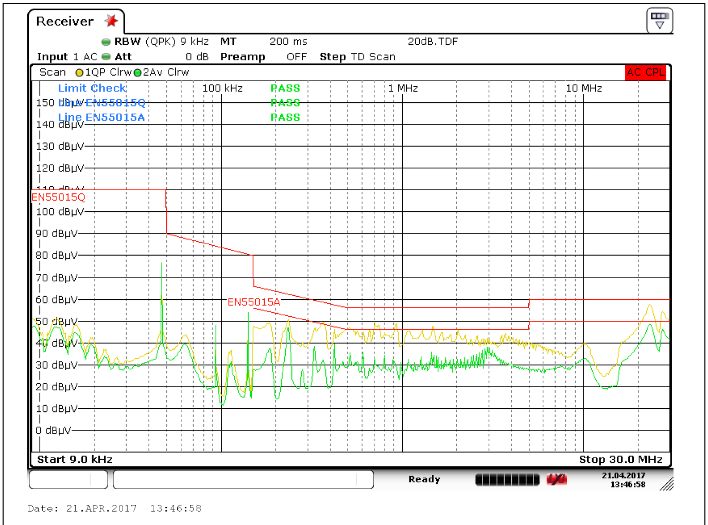
Figure 18 Conducted EMI measurement according to EN 55015
