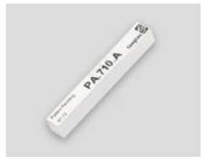
The Warrior, is a revolutionary patentpending, high-efficiency SMD ceramic antenna. This mighty, but small (40×5×6 mm) wideband 4G/3G/2G antenna, operates at 698MHz to 960MHz and 1710MHz to 2690MHz. The exceptional wide-band response means it's the ideal antenna for all LTE applications that also need highefficiency and backward compatibility
