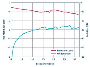
Figure 6. SPDT MEMS switch performance, QFN packaged.
