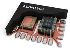
Figure 1. ADI MEMS switch technology.
