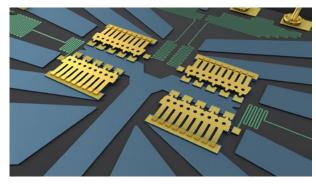
Figure 4. Close-up graphic showing four MEMS cantilever switch beams (SP4T configuration).
