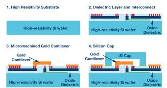
Figure 3. MEMS switch fabrication overview.
