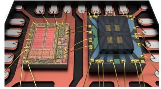
Figure 5. Drive IC (Left), MEMS switch die (Right) mounted on and wire bonded to a metal lead frame.
