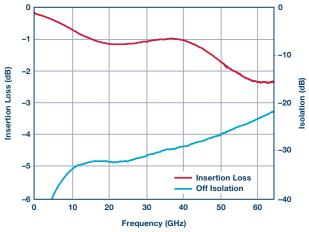
Figure 7. SPST MEMS switch performance, on die probed measurement.
