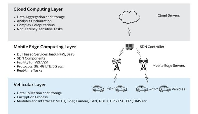
**The Cloud Layer**: is where enormous volumes of data are stored, aggregated, and processed. It is also here that more complex computation takes place. The cloud is ideal for longer-term storage in which latency is not critical to applications
