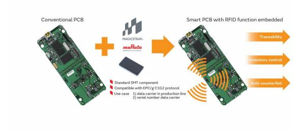
The retailing industry is the main area of application of the RFID solutions. The RFID of Murata is very small in size and could be easily embedded into luxury items or jewels for verifying the source of the merchandise, which helps to prevent counterfeit items. In general, the retailers and warehouse dealers use a barcode or QR code on
