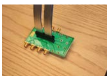
Wire-to-board test board for high-speed test
