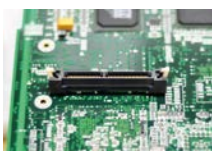
80 pos. connector in high-speed application (PCIe)
