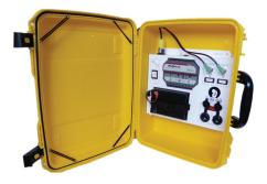
Advanced solar controller, ports and plugs, in watertight and dust-proof high-quality suitcase, made to hold up in harsh environments. System contains an integrated 12V, 12.8Ah battery, which is charged by a solar panel. Suitcase has 2 WCS Lighting Connectors, two 12VDC Accessory (lighter) Sockets, and two Expansion Ports to allow for optional accessories. A homerun cable and installation hardware are included.
