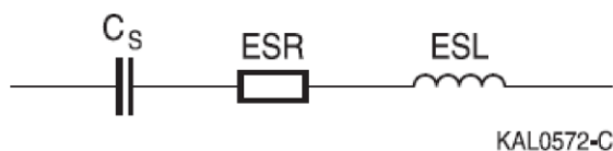
Figure 4: Equivalent circuit of a real capacitor (Source: TDK)
