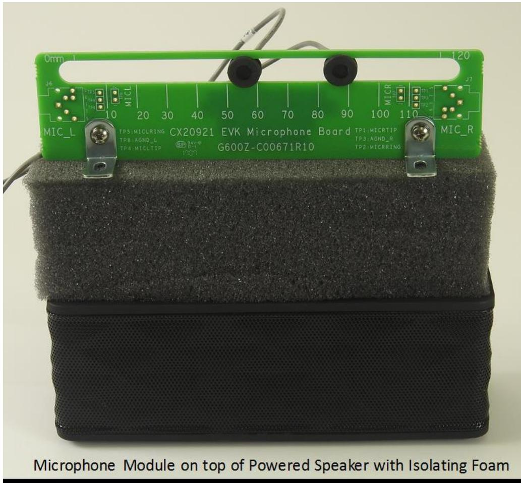
Microphone Module on top of Powered Speaker with Isolating Foam
