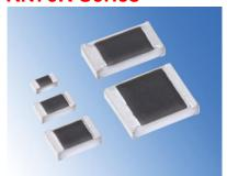
With a T.C.R. down to  $\pm 5$  ppm and a tolerance as low as  $\pm 0.05$  % the new RN73R series from KOA is ideal for high precision circuits in various industrial and measuring applications.
