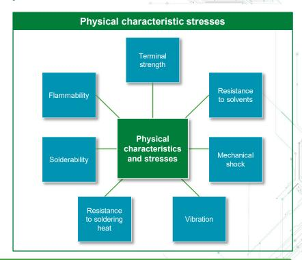
Two main tests: Environment stresses and physical characteristics stresses
