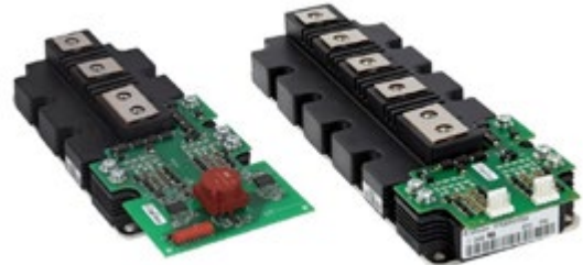
Figure 5: Dual-Channel driver 2ED250E12_F and booster stage MA300E17 mounted to the according power module
