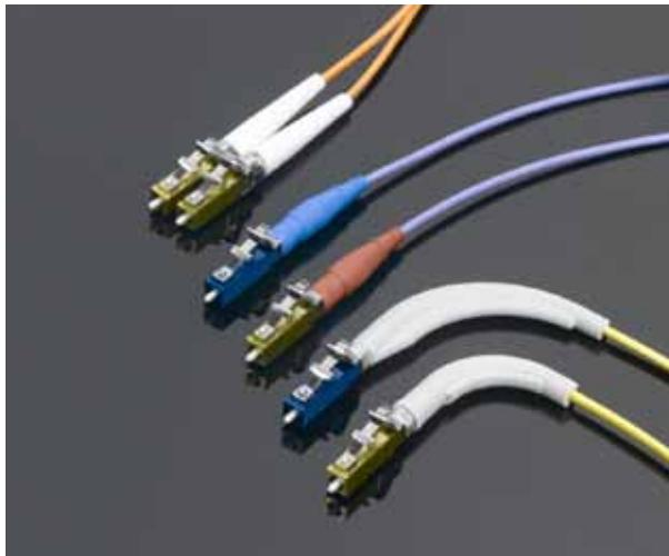
*Metal-housing LC2+ connectors, such as those shown (above), offer a high-performance, discrete-fiber interconnect solution for use in severe operating environments such as those encountered by military vehicles. LC2+ interfaces are found on many active military LED and laser-based devices, and they support enhanced performance aerospace-grade optical cabling. LC2+ connectors also meet all FOCIS 10 specifications.*
